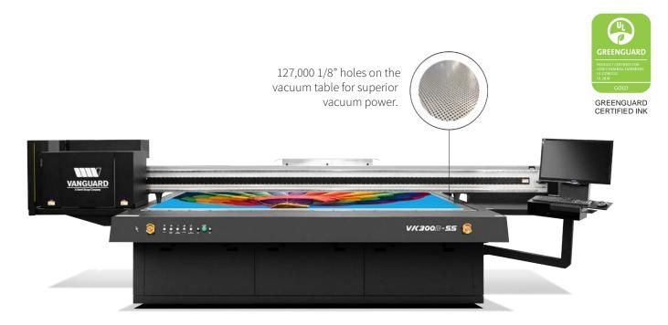
The VK300D-SS features an upgraded robust vacuum table. Built with a custom milled aluminum vacuum table designed specifically to pull down the most warped substrates. The VK300D-SS reduces the risk of head strikes and offers you peace of mind when printing severely warped materials. The vacuum table is made up of 127,000 1/8th inch holes and two 5 horsepower Spencer blower motors for maximum substrate stability while printing.
