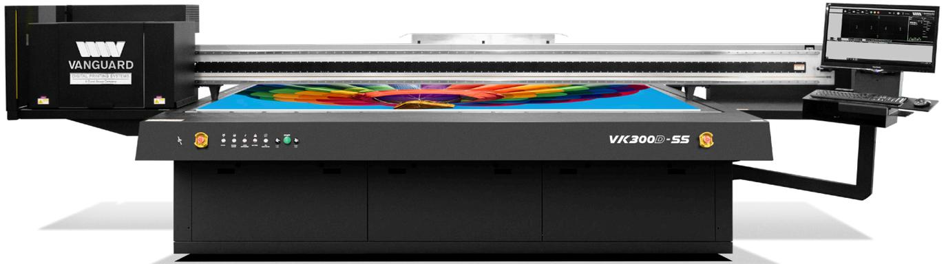
The VK300D-SS features an upgraded high-suction, robust vacuum table. Built with a custom milled aluminum vacuum table designed specifically to pull down warped substrates, the VK300D-SS reduces the risk of head strikes and offers you peace of mind when printing severely warped materials. With the capability to digitally print and decorate difficult materials like wood, the VK300D-SS is the ultimate tool for your workshop, and the only limitation is creativity.
